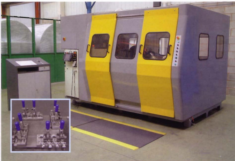
The IC-Flexible Grinding System. The robotic system uses a multi position jig plate (see inset).
